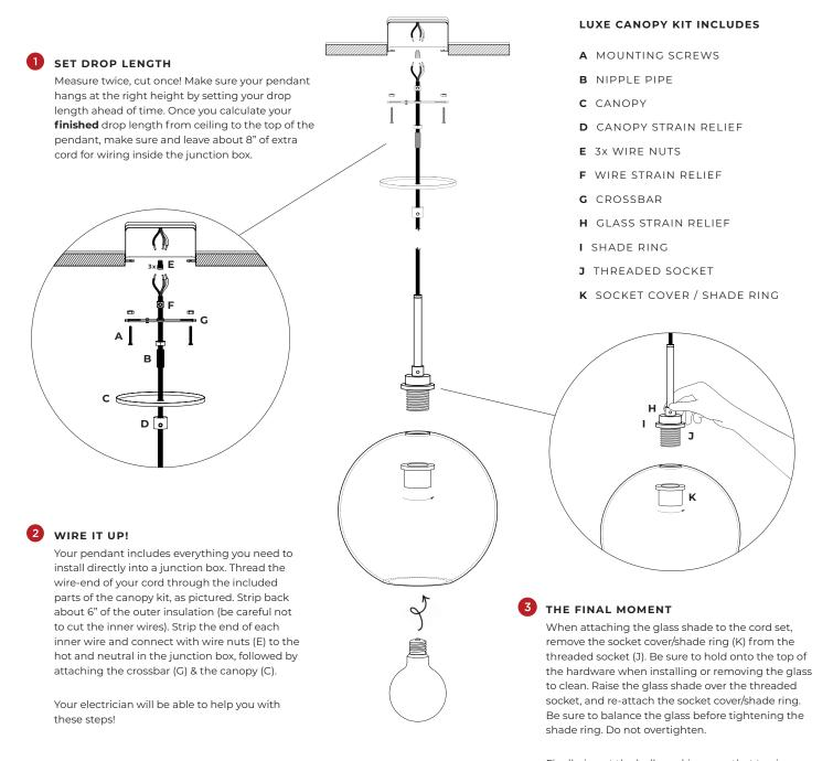
Finally, insert the bulb, making sure that too is straight. Turn the circuit breaker back on, flip the switch, and prepare to be illuminated!
